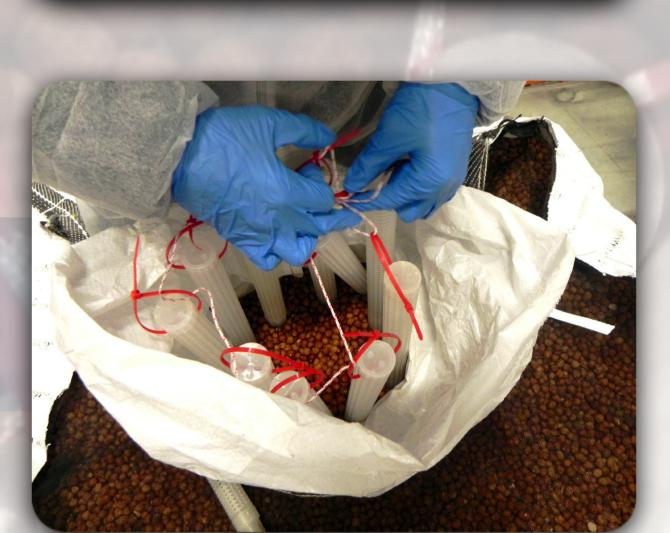
**APPLICATION** - The test started when the  $N_2$  saturation reached 99,9%. After **21 days** of complete and constant  $N_2$  saturation, the desaturation process started. During the whole period of the test, the temperature and % saturation by  $N_2$  were constantly monitored and kept.
